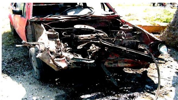
Golf Mk1 vehicle after 130mm projectile explosion, at an angle of 62° - photograph PICTO754
