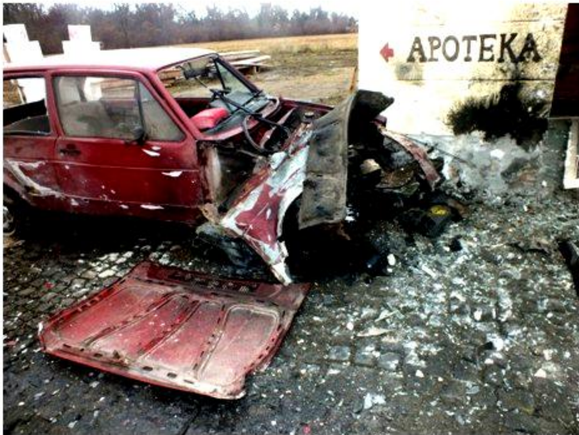
Experimental car, after 130mm projectile explosion
