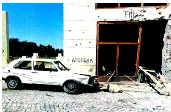
Golf Mk1 vehicle after 130mm projectile explosion at an angle of 20° from the East - second experiment by former defense expert
