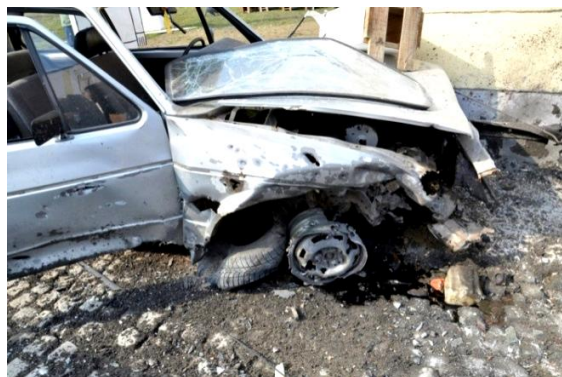
Golf Mk1 vehicle after 130mm projectile explosion at an angle of 62° - photograph from 12 March 2015
