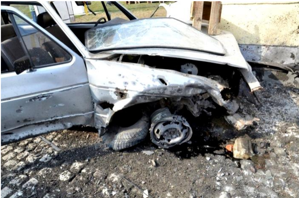
Appearance of front right part of the second vehicle after experimental explosion
