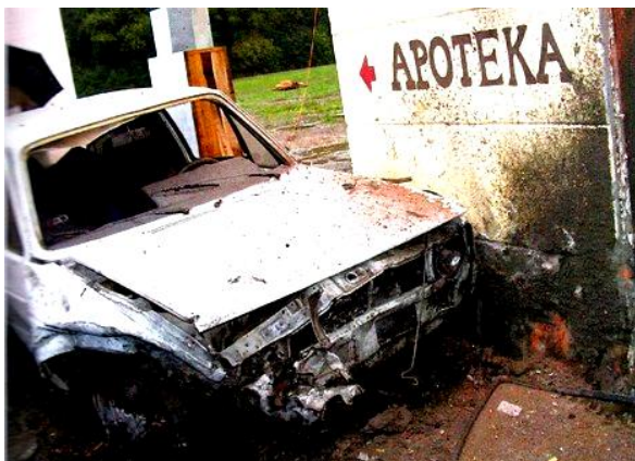
Golf Mk1 vehicle after 130mm projectile explosion at an angle of 62° - photograph from 04 September 2014
