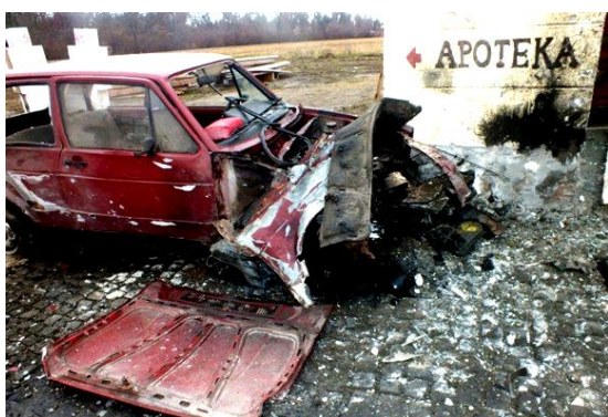
Golf Mk1 vehicle after 130mm projectile explosion at an angle of 62° - photograph from 10 February 2016
