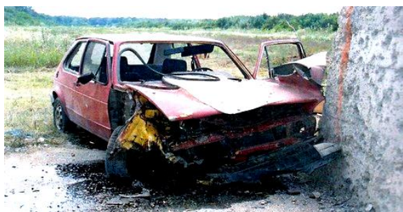
Golf Mk1 vehicle after 130mm projectile explosion, at an angle of 62° - photograph PICTO754
