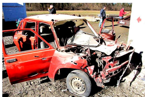
Zastava 101 vehicle after 130mm projectile explosion at an angle of 50° from South-East - from 11 February 2016, experiment by J. Sharon
