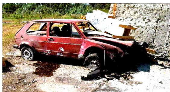
Golf Mk1 vehicle after 130mm projectile explosion at an angle of 62° - photograph DSCN5605
