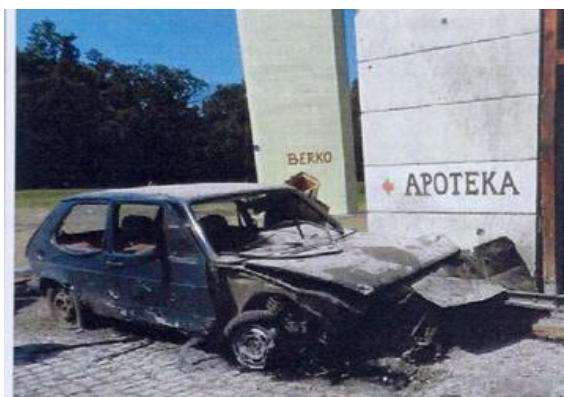
Golf Mk1 vehicle after 130mm projectile explosion at an angle of 62° - photograph from 25 August 2014
