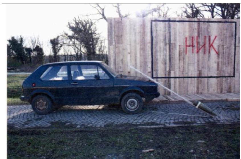
Figure 11— Determining the minimum angle of descent according to the findings of the Tuzla CSB
