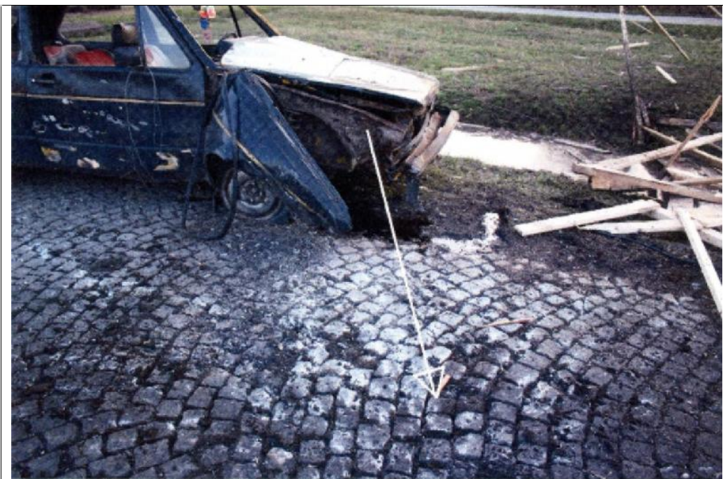
Figure 22 — The centre of the explosion of the projectile that was placed at an angle of 64^{\circ}50' . The tip of the arrow indicates the spot where the tip of the projectile was before the explosion — general view
