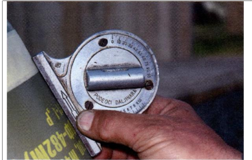
Figure 15 — Measuring the projectile’s minimum angle of descent of 62°
