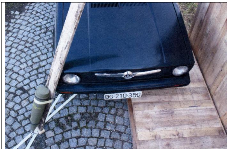
Figure 14 — Position of the Golf 1 in the case of a minimum angle of descent of 62°
