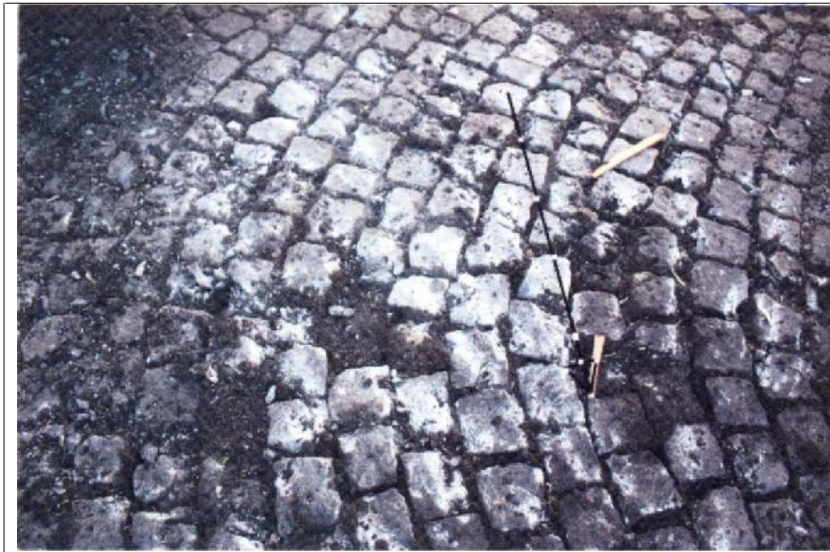
Figure 21 — The centre of the explosion of the projectile that was placed at an angle of 64^{\circ}50' . The tip of the arrow indicates the spot where the tip of the projectile was before the explosion
