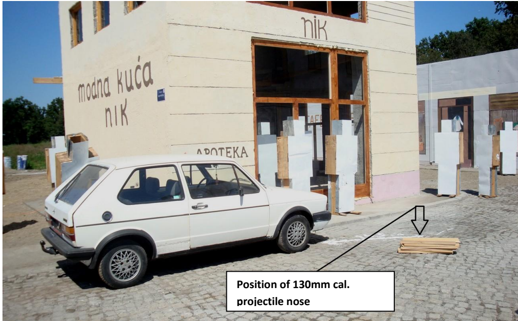
Figure 3 – Appearance of the site with the car and dolls in approximate positions as they were before the explosion, with marked position of projectile nose
