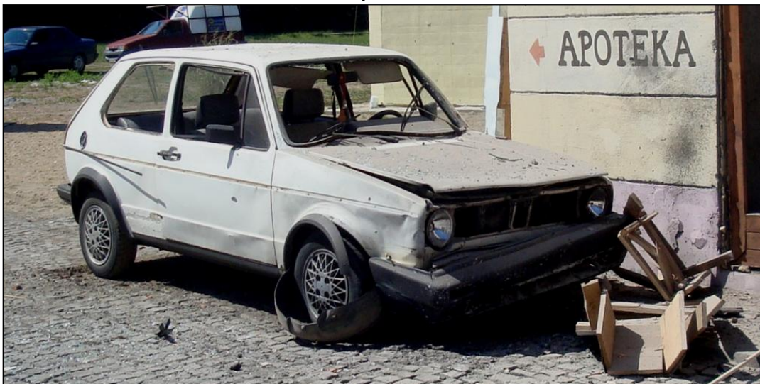
Figure 24 – Appearance of the "GOLF 1" car used during experimental projectile explosion, with visible consequences of the explosion
