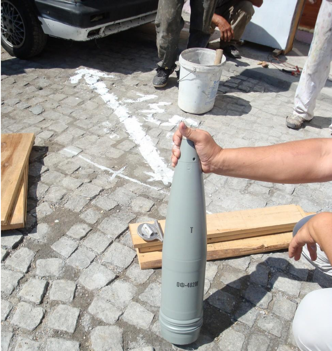
Figure 6 – Appearance of 130mm caliber projectile OF-482M immediately before setting it up in the position for activating, thick white line marks the direction of the projectile towards the car
