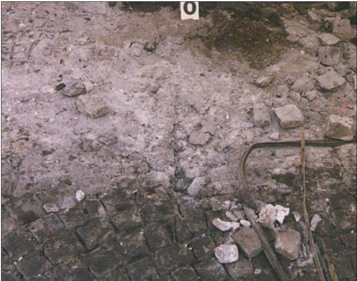
Figure 22 – Appearance of furrow made by fuze or some other metal object with ground moving traces from granite cubes, dust or sand
