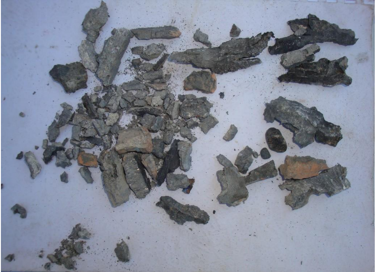
Figure 16 – Pieces of projectile body, found on the ground on the right side of "NIK store" model facade
