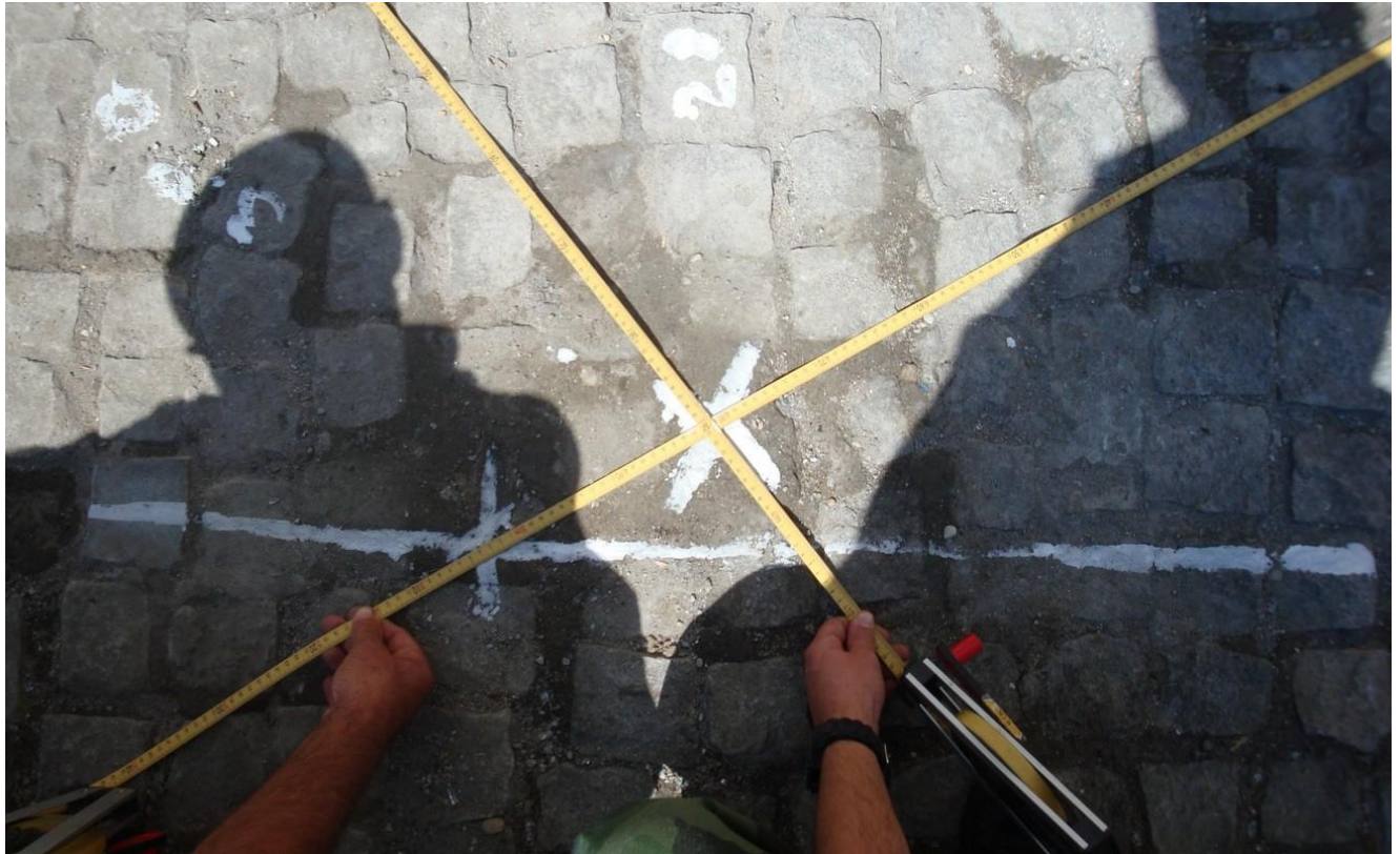
Figure 5 – Defining of spot, i.e., the position of projectile nose in relation to the "NIK" store object, based on the sketch of the crater No.: 20-1/02-3-9-7-175/95
