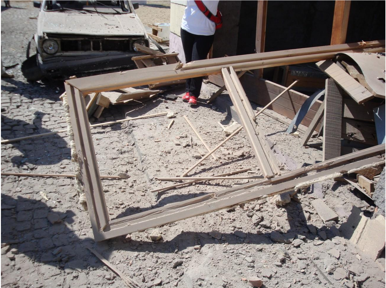
Figure 10 – Appearance of remains of the dolls, set up in front of "NIK" store object, after the explosion, with ripped-out frame of shop door
