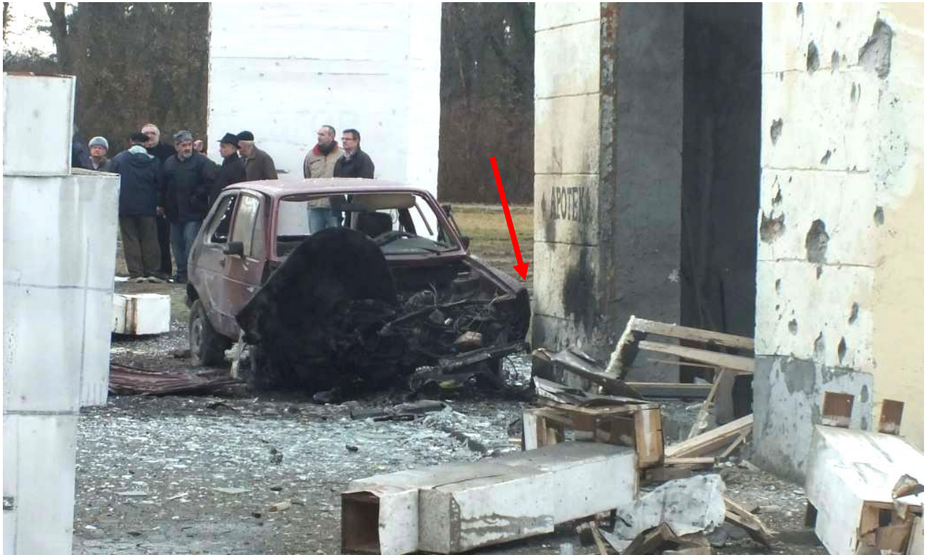
Photo showing that the car was moved sideways by the blast
