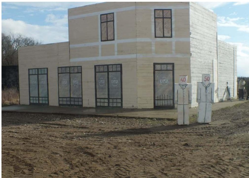
Across the square (36 m from burst point, café Kapija was virtually untouched by fragments during the experiment,
