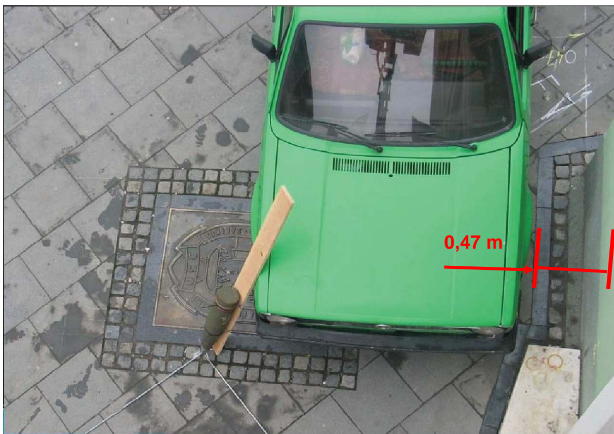
Reconstruction of a 130 mm incoming projectile arrival with AoF = 62° (as positioned by Prof. Berko ZECEVIC)
